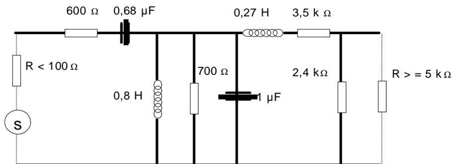
**Figure 2: Filter circuit**
