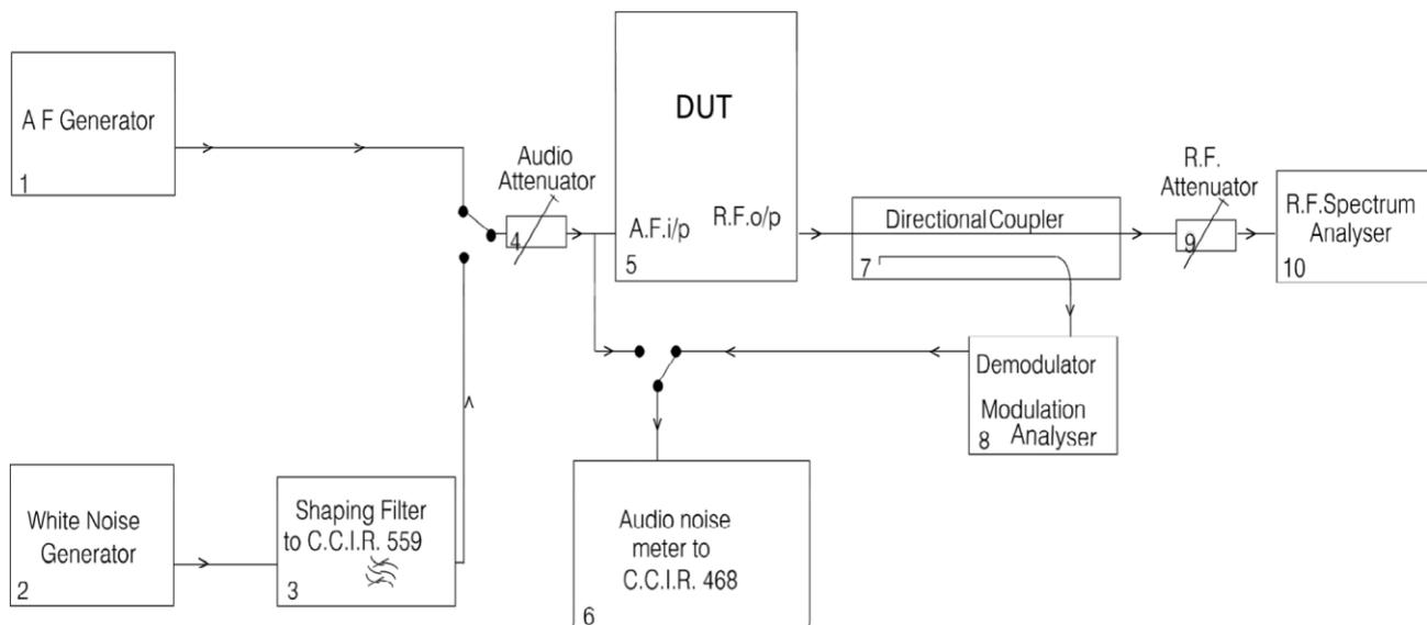
**NOTE:** If the DUT incorporates ancillary coding or signalling channels, for example, pilot tone, etc. these should be switched on prior to measuring the transmitter RF output spectrum.
