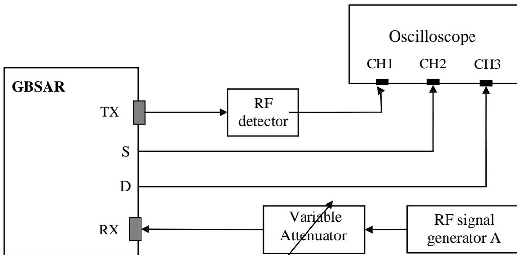
**Figure F.1: DAA measurement arrangement**
