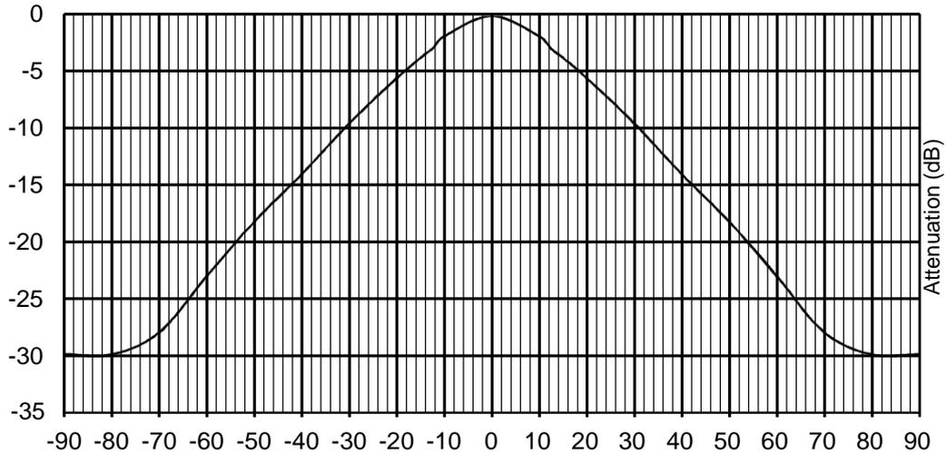
**Figure F.7: Minimum attenuation of the vertical antenna pattern**
