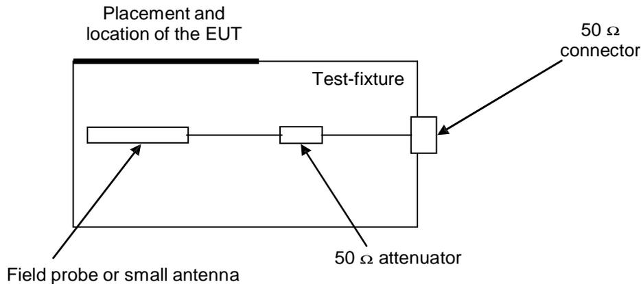
**Figure 4: Test fixture**
