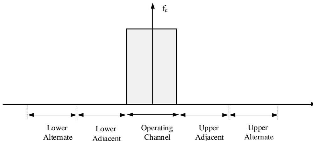
**Figure 1: Adjacent and alternate adjacent channel definitions**
