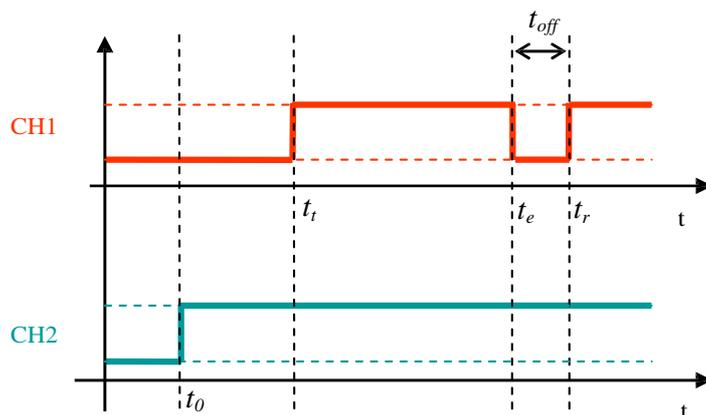
Figure F.5: Maximum transmit off time,  $t_{off}$  measurement
