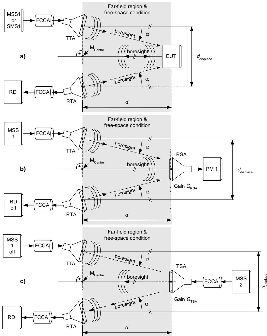
**Figure B.9: Measurement arrangement with two test antennas:**
