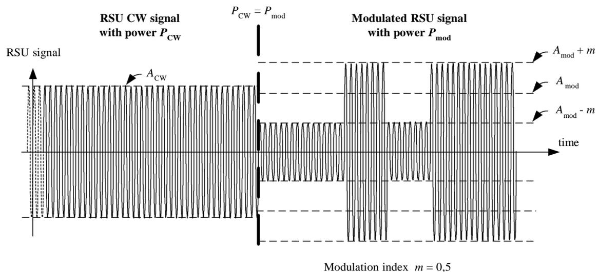
**Figure B.15: RSU transmit signal**
