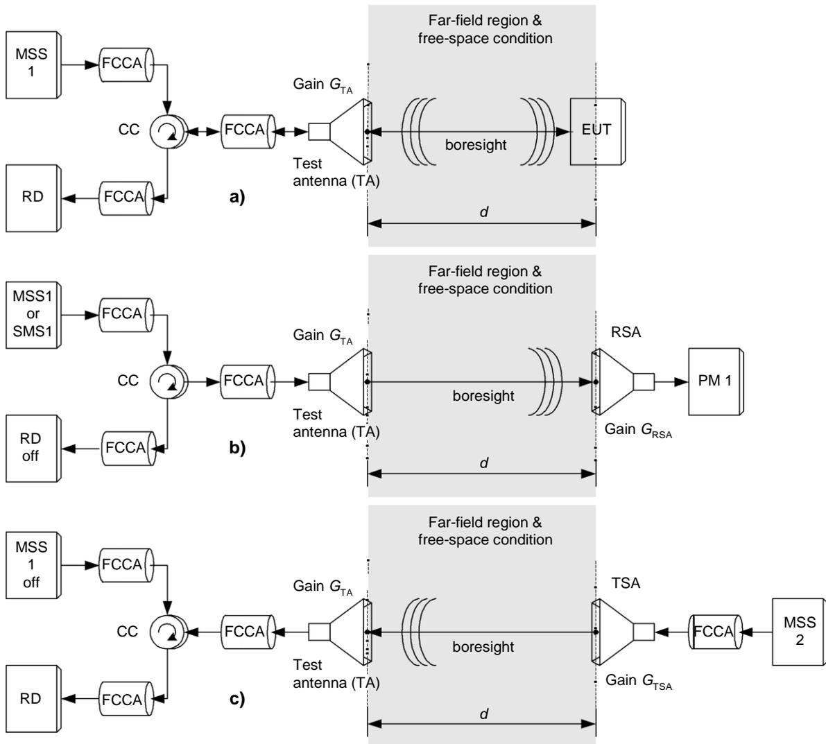
**Figure B.8: Measurement arrangement with one test antennas:**
