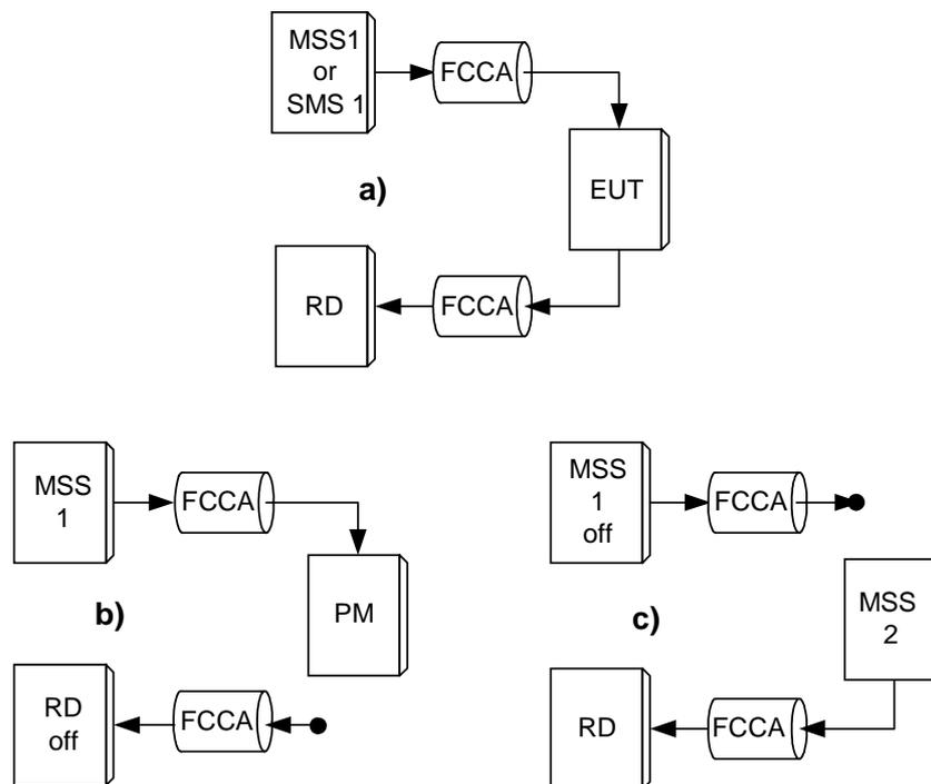
**Figure B.7: Measurement arrangement with two antenna connectors:**
