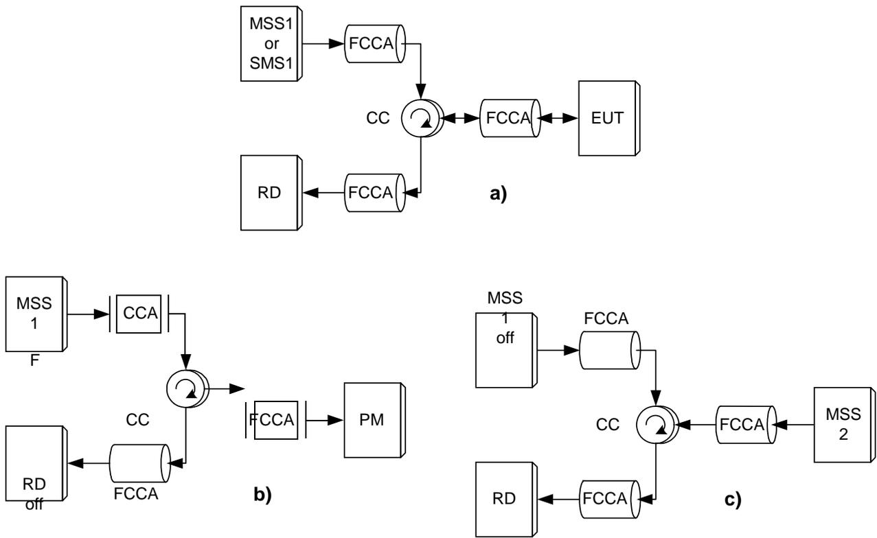
**Figure B.6: Measurement arrangement with one antenna connector:**
