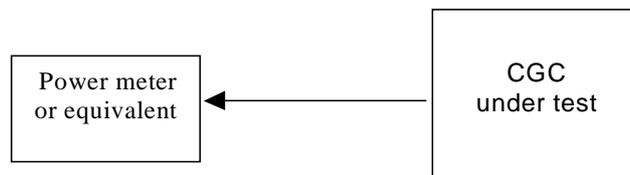
**Figure D.1: Measuring system Set-up for maximum output power, total power dynamic range**
