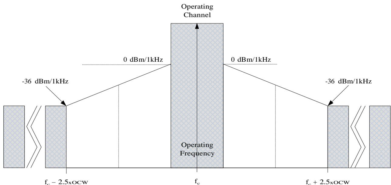
**Figure 4: Out-of-Band Domain for Operating Channel**
