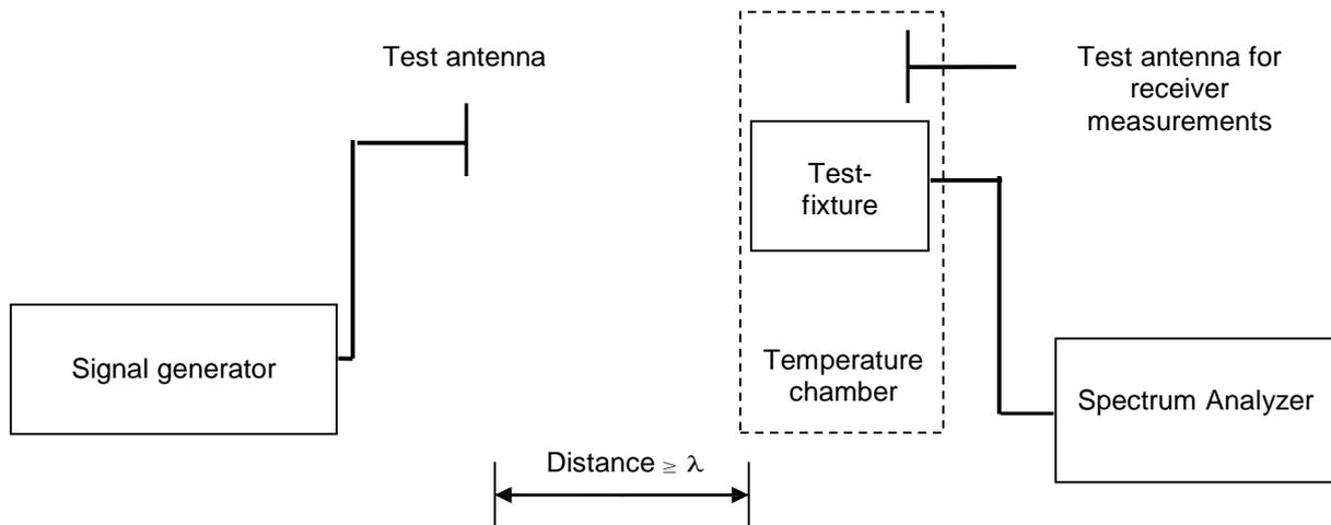
**Figure C.2: Validation of test set-up without EUT**
