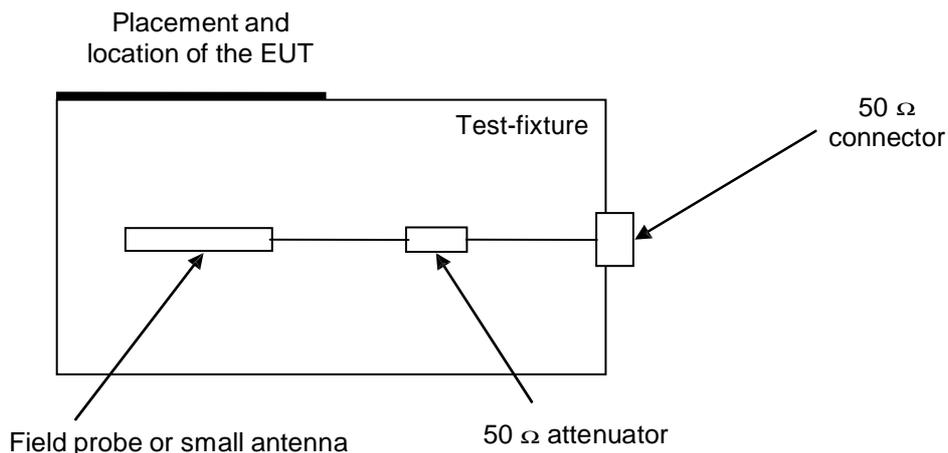
**Figure C.1: Test fixture**
