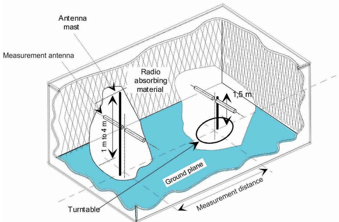
**Figure B.2: A typical Semi Anechoic Room**
