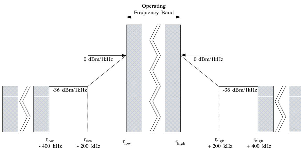
**Figure 5: Out-of-Band Domain for Operating Frequency Band**
